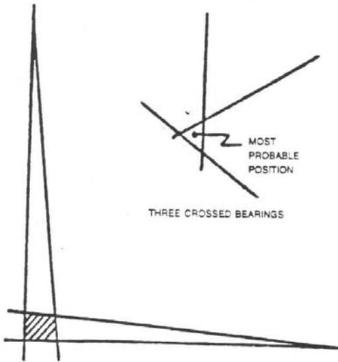
RIGHT ANGLE CROSSED BEARINGS, FIVE DEGREE READING ERROR
